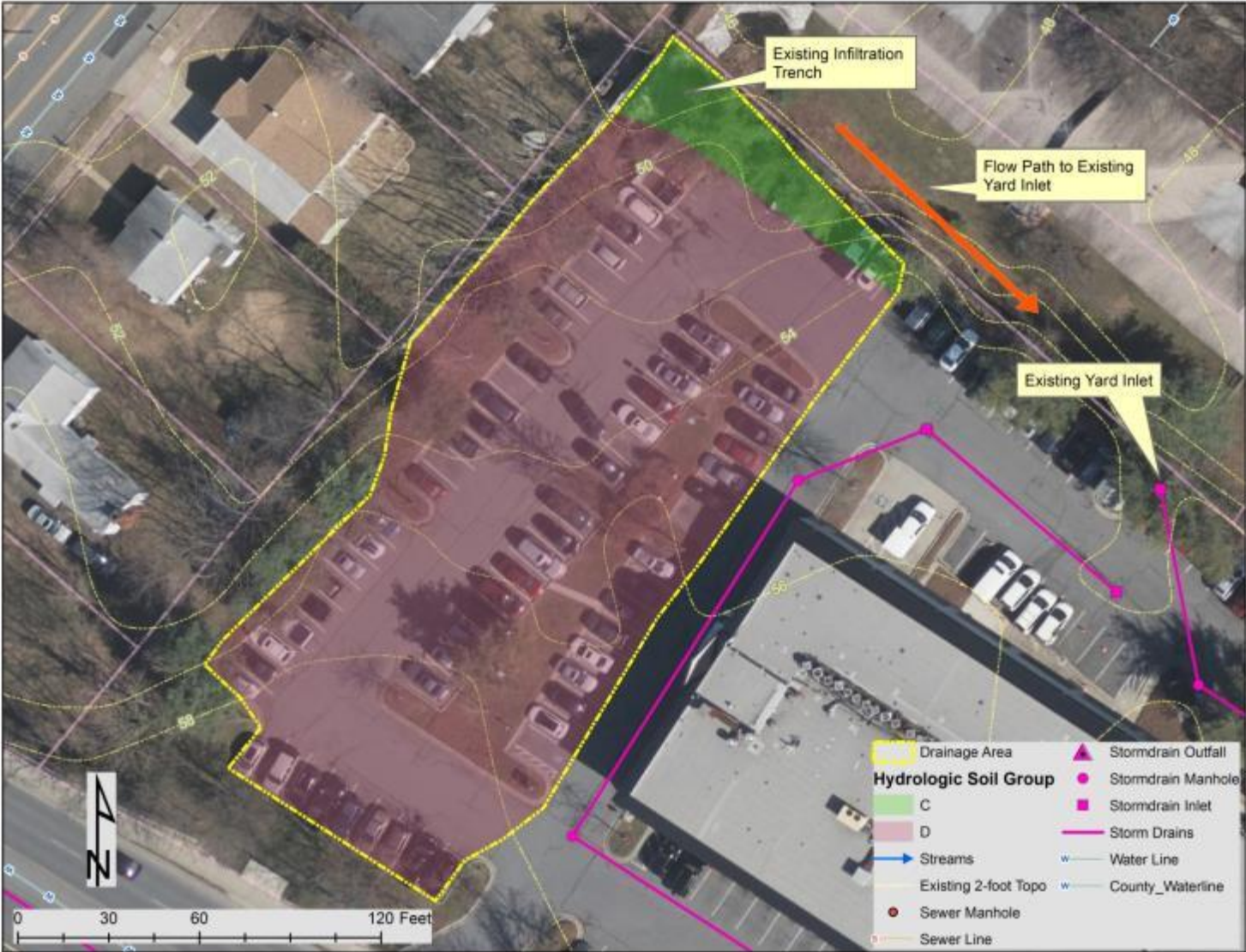
Figure 22: Existing Conditions and Drainage Area
