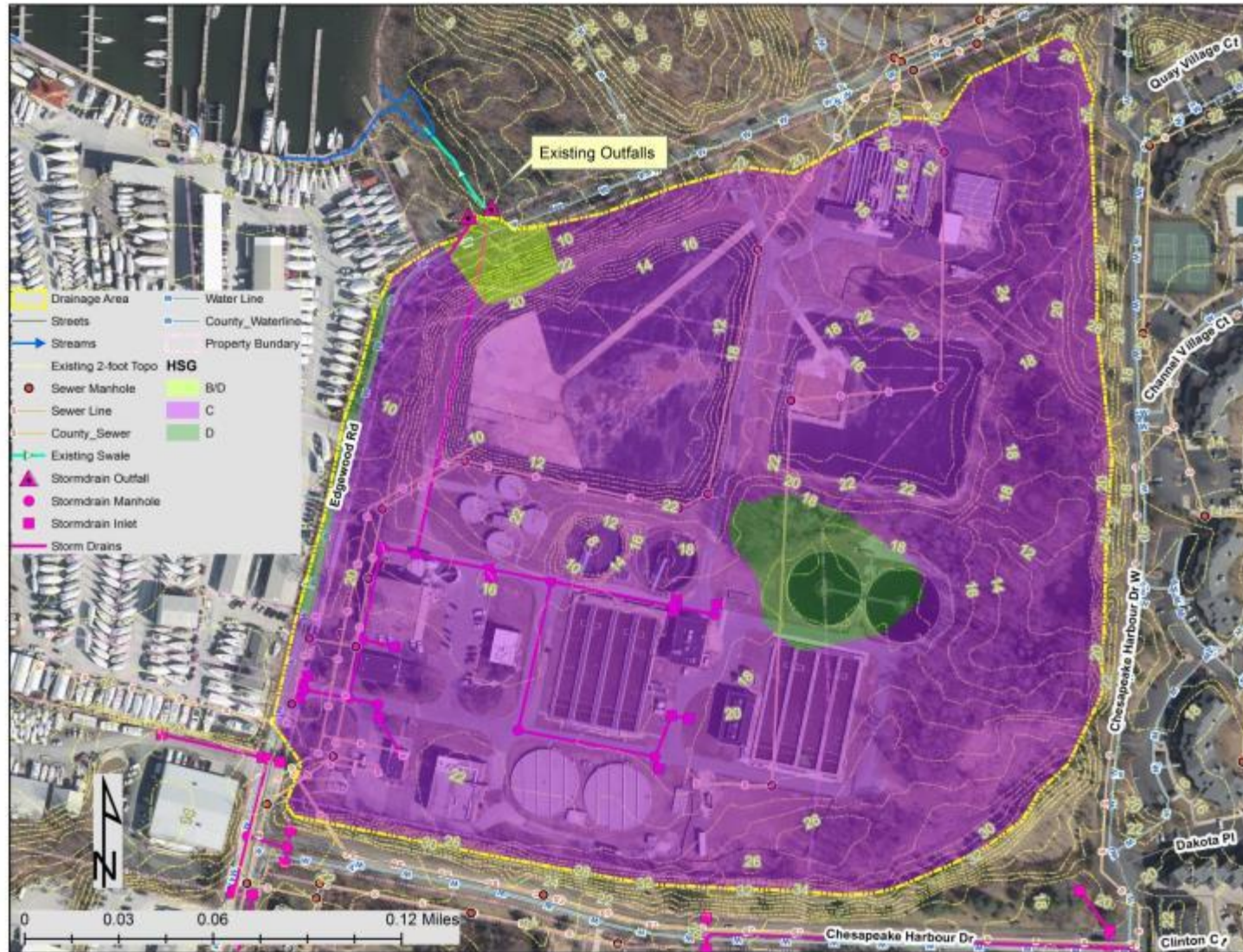
Figure 43: Existing Conditions and Drainage Area
